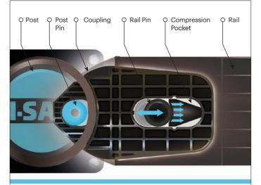
**PHASE 1:** Memaplex<sup>™</sup> rail flexes to absorb impact, initiating the rail pin to slide forward and transfer load energy to the compression pocket.
